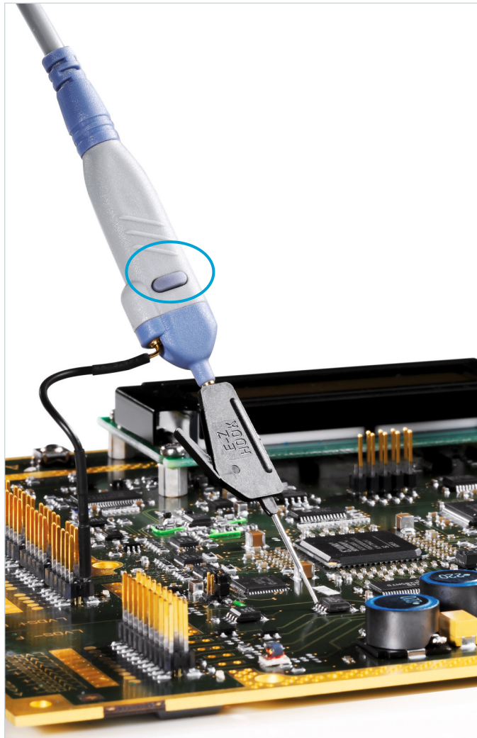
Practical design: micro button for convenient instrument control. Diverse probe tips and ground cables are included as standard accessories.
