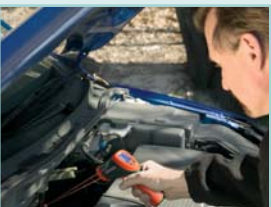
Max hold indicates and holds the peak temperature for easy identification of hot spots
