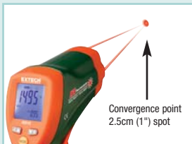
Two laser points converge at a distance of 76.2cm (30") and form a 2.5cm (1") spot.
